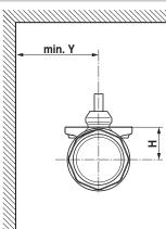
X/Y: Minimum distance with respect to the valve centre.
